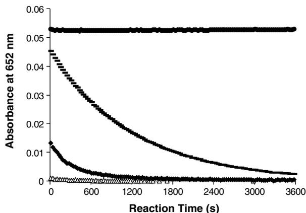
**Figure 2.** Plot of absorbance (652 nm) versus time of Lu(III)–AAIII (●), NETA (◆), DOTA (○), and DTPA (Δ) at pH 4.5 (0.15 M NH<sub>4</sub>OAc) and 25 °C.
