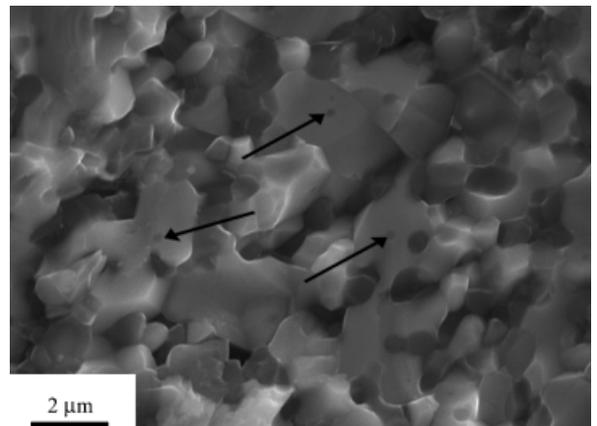
Fig. 4. Scanning electron micrograph from a fracture of the as-sintered composite (examples of intragranular SiC particulates are marked with black arrows).
