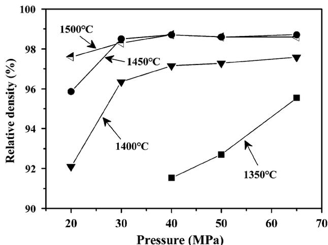
Fig. 2. Variation of relative density depending on the sintering temperature and pressure.
