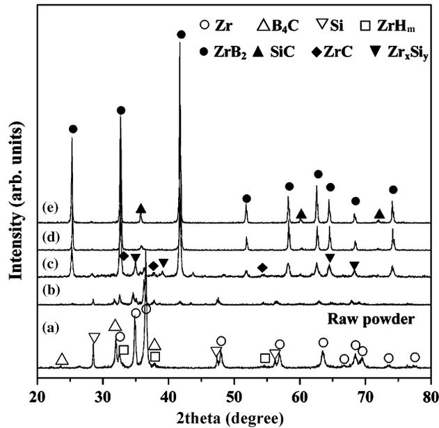
Fig. 1. X-ray diffractometry patterns of the Zr/Si/B<sub>4</sub>C mixed powders heated at (b) 900°C, (c) 1000°C, (d) 1200°C, and (e) 1500°C.
