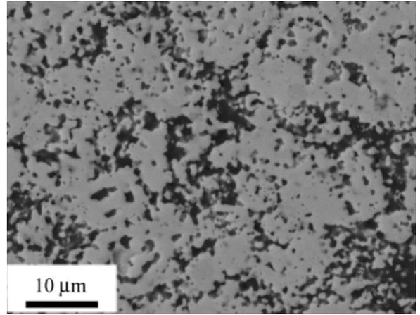
Fig. 3. Backscattered electron image of a polished surface of the as-sintered composite (the gray phase represents ZrB<sub>2</sub>, and the dark phase represents SiC).
