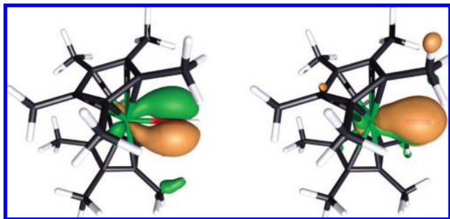
Figure 10. Ti–O \pi -bonding in the collinear 7 arising from interaction of d_{xy} and p_y orbitals (left) and d_{xz} and p_z orbitals (right). Both molecular orbitals are doubly occupied. Orbital contours are plotted at the 5% probability level.
