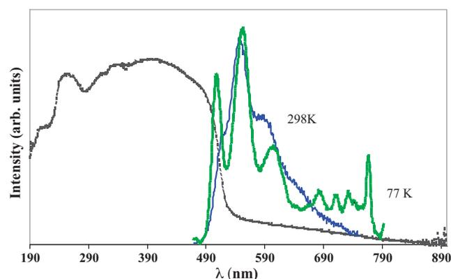
**Fig. 5.** Photoluminescence spectra of the polymer measured at 298 and 77 K. The excitation wavelength was 300 nm and 350 nm respectively. The emission peaks occur at: (298) 517, 548 and 590 nm; (77 K) 526, 567, 616 nm.
