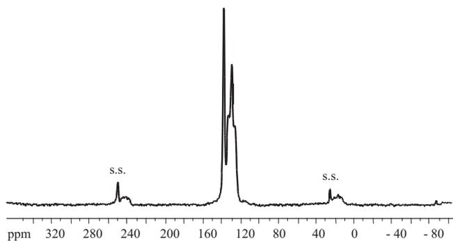
**Fig. 4.** CPMAS spectrum of polycondensation product of (*E*)-[1-(4-bromophenyl)-2-(1,1,3,3,3-pentamethyldisiloxy)]ethene made at r.t., s.s. denotes spinning sidebands.
