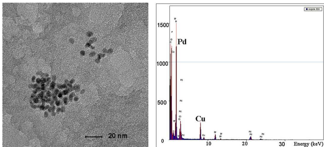
**Fig. 2.** TEM micrograph and energy dispersive X-ray spectrum (with the use of Cu grid) of post reaction solution between (*E*)-[1-(4-methylphenyl)-2-(1,1,3,3,3-pentamethyldisiloxy)] ethene (**1e**) and bromobenzene.
