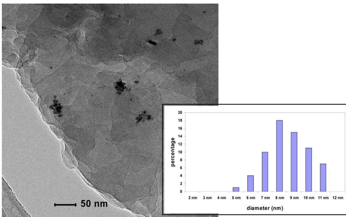
**Fig. 3.** TEM micrograph of polycondensation product of (*E*)-[1-(4-bromophenyl)-2-(1,1,3,3,3-pentamethyldisiloxy)]ethene (**1d**) and the corresponding size histogram of Pd(0) nanoparticles (70 Pd nanoparticles measured).
