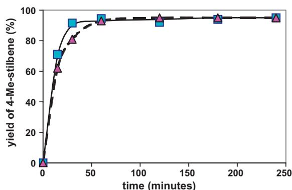
**Fig. 1.** Reaction profile study of the Hiyama cross-coupling of (*E*)-[1-(4-methylphenyl)-2-(1,1,3,3,3-pentamethylidisiloxy)]ethene (**1e**) with bromobenzene (solid line), and a poisoning test (dotted line) with Hg(0) added before reaction starts (reaction conditions: DMF, 140 °C).
