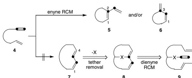
Scheme 1. Generation of disubstituted 1,3-dienes by ring-closing metathesis.
