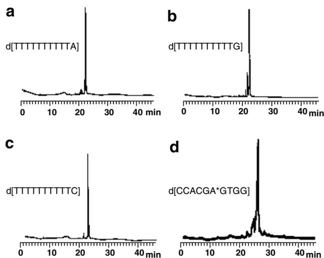
Figure 3. Anion-exchange HPLC profiles of the crude mixtures obtained using the activated phosphite method under the conditions used for ABI 392 DNA synthesizer. (a) d[TTTTTTTTTTA], (b) d[TTTTTTTTTTTG], (c) d[TTTTTTTTTTTC], and (d) d[CCACGA\*GTGG], A\* = ac<sup>6</sup>az<sup>8</sup>c<sup>7</sup>A.
