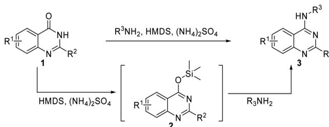
**Scheme 1.** One-pot synthesis of 4-aminoquinazolines mediated by HMDS.
