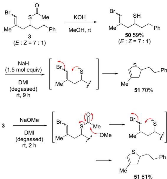
used directly instead of thiol **50** for this intramolecular substitution reaction. As expected, treatment of thioacetate **3** with 1.5 mol equiv of NaOMe at room temperature in DMI gave dihydrothiophene **51** in 61% yield (Scheme 14).
