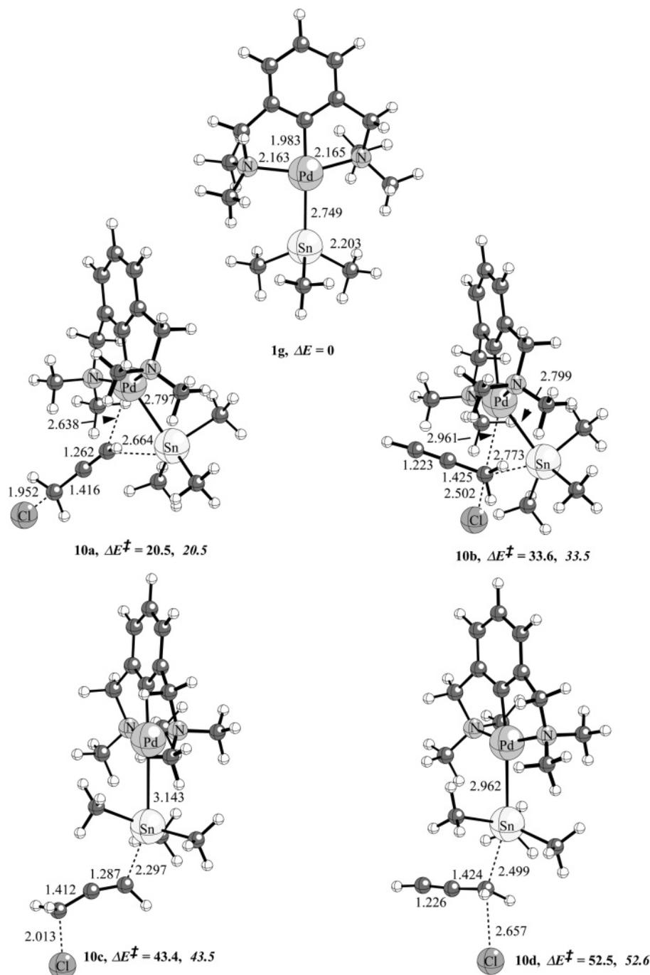
**Figure 2.** Calculated geometries for **1g** and the TS's of the trimethylstannane transfer reaction. The ZPV-corrected energies are given in italics. Energies in kcal mol<sup>-1</sup> and bond lengths in Å.
