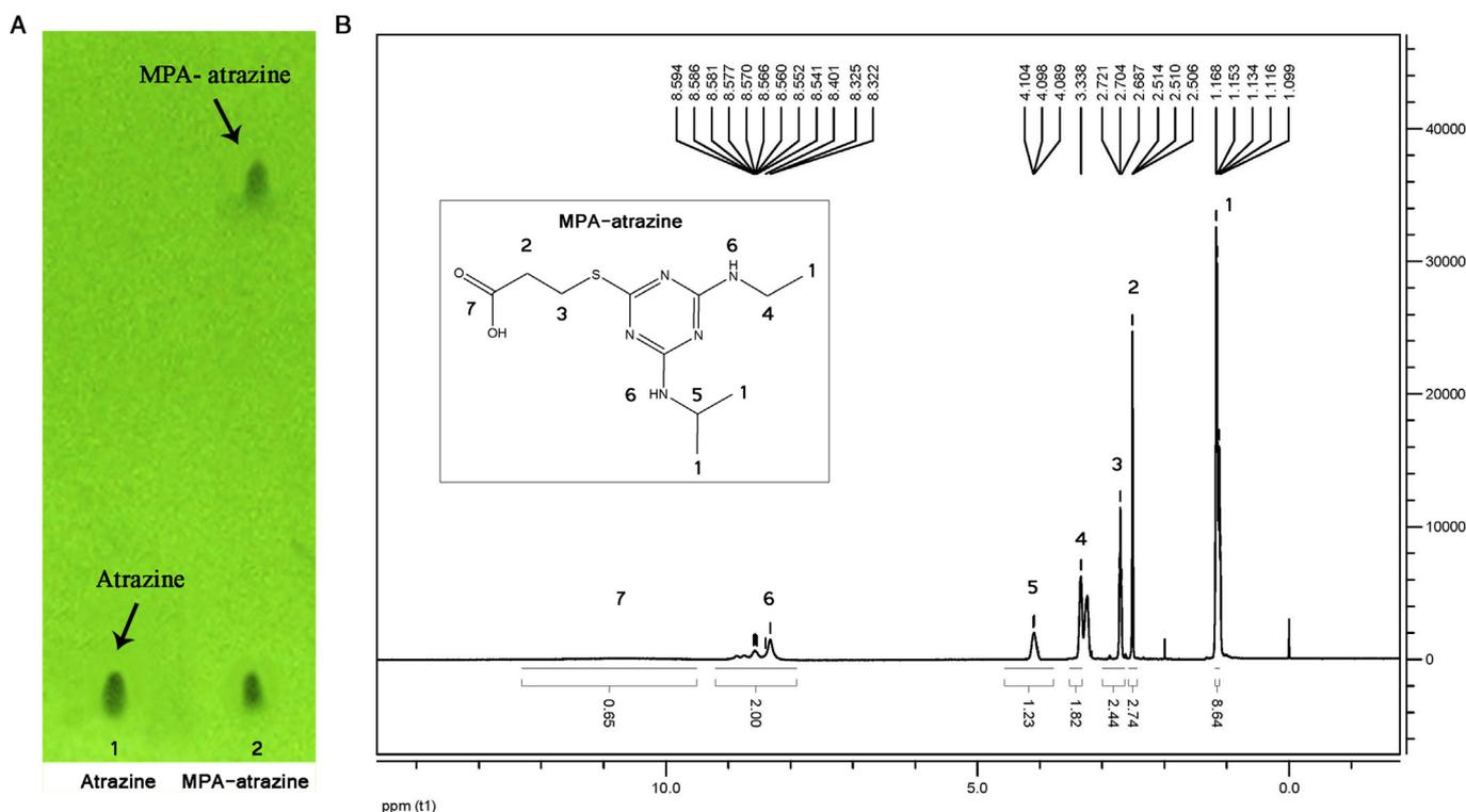
Fig. 2. The verification of MPA-atrazine: a) TLC of MPA-atrazine. Compared with atrazine original drug, there was new product (MPA-atrazine) generated; b) <sup>1</sup>H NMR spectrum of MPA-atrazine. The inset showed details of the fine peaks corresponding to some of MPA-atrazine.
