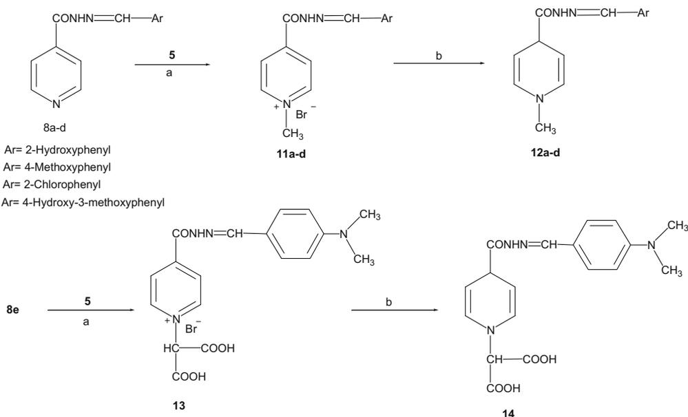
**Scheme 3.** Synthesis of *N*-methyl PCDSs derivatives **12a–d** and MPCDS **14**. Reagents: (a) EtOH, reflux; (b)  $\text{Na}_2\text{S}_2\text{O}_4$ ,  $\text{NaHCO}_3$ ,  $\text{CH}_2\text{Cl}_2$ ,  $\text{N}_2$  gas.
