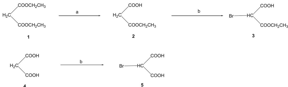
Scheme 1. Synthesis of bromomalonate derivatives **3** and **5**. Reagents: (a) KOH, EtOH, HCl; (b) Br<sub>2</sub>, HOAc.
