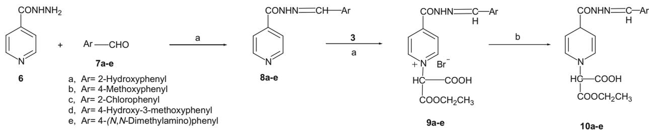
**Scheme 2.** Synthesis of MEPQDSs **10a–e**. Reagents: (a) EtOH, reflux; (b)  $\text{Na}_2\text{S}_2\text{O}_4$ ,  $\text{NaHCO}_3$ ,  $\text{CH}_2\text{Cl}_2$ ,  $\text{N}_2$  gas.
