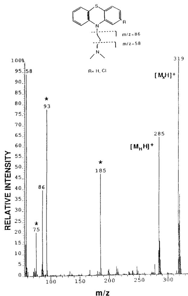
Figure 1. Positive liquid secondary ion mass spectrum of chlorpromazine in glycerol (0.037 M). Asterisks denote matrix peaks.
