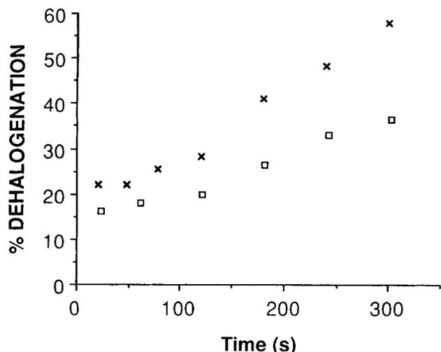
**Figure 6.** Percentage dehalogenation of chlorpromazine (0.0068 M in glycerol) at different beam densities as a function of time of analysis. Beam density: (□) 0.027; (×) 0.042  $\mu\text{A mm}^{-2}$ .
