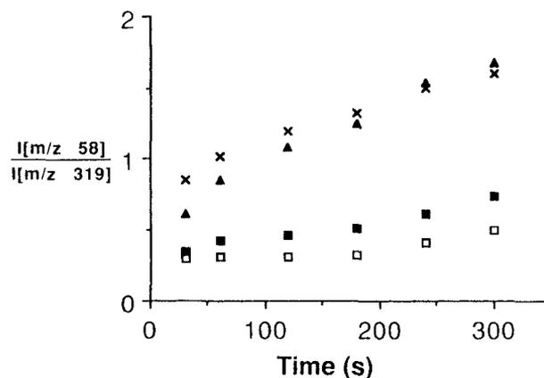
Figure 3. Ratio of relative intensity of the amino side-chain fragment  $m/z$  58 peak to the intensity of the protonated molecular ion  $m/z$  319 peak as a function of time of analysis and concentration. Concentration: (□) 0.0068; (■) 0.011; (▲) 0.037; (×) 0.097 M.
