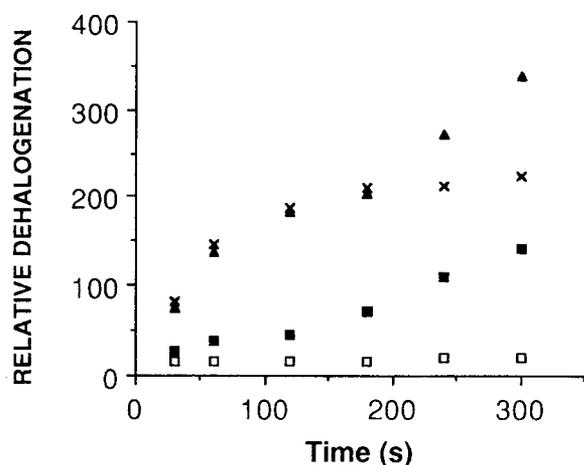
**Figure 4.** Relative dehalogenation of chlorpromazine at various concentrations in glycerol as a function of time of analysis. Concentration: (□) 0.0068; (■) 0.011; (▲) 0.037; (×) 0.097 M.
