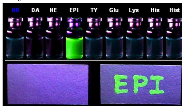
Figure 3 Fluorescence responses of (A) sensor NB ( 1 \times 10^{-5} M) in 1:9 v/v DMSO:phosphate buffer at 0.01 M, pH 7.4) in the presence of the various guests 100 equiv. and Fluorescence images (B) of (a) sensor NB and (b) The filter paper dipped in sensor NB solution, and the word "EPI" with EPI solution was exposed to the UV light.
