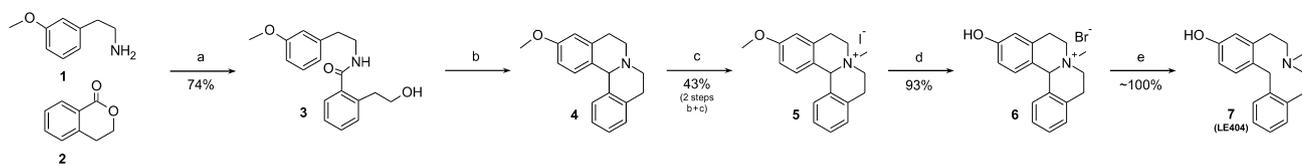
**Scheme 1.** Reagents and conditions: a) KCN, 70 °C, 7 d; b) phosphoryl chloride, MeCN, 0 °C to rt, reflux 24 h; c) methyl iodide, MeCN, reflux, 48 h; d) boron tribromide, chloroform, 0 °C to rt, 24 h; e) Na<sup>0</sup>, liq. ammonia, -78 °C to rt, 12 h.
