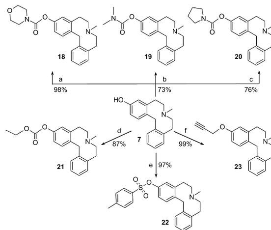
**Scheme 3.** Reagents and conditions: a) 4-morpholine-carbonylchloride, NaH, DCM, 0 °C to rt, 24 h; b) dimethylcarbamoyl chloride, NaH, DCM, 0 °C to rt, 24 h; c) 1-pyrrolidinecarbonyl chloride, NaH, DCM, 0 °C to rt, 24 h; d) ethyl chloroformate, NaH, DCM, 0 °C to rt, 3 h; e) toluene-4-sulfonic acid chloride, NaH, THF/DCM (3:1), 0 °C to rt, 2 h; f) propargyl bromide, NaH, toluene/DMF (1:1), 0 °C to rt, 1 h.
