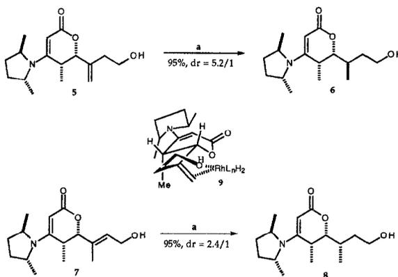
**Scheme 3:** Rh(1,4-DIPHOS)(NBD)<sup>+</sup>BF<sub>4</sub><sup>-</sup>, CH<sub>2</sub>Cl<sub>2</sub>, H<sub>2</sub> (650 psi)
