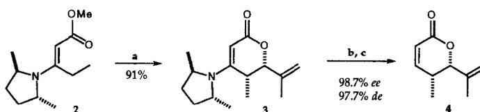
**Scheme 2:** (a) (1) LDA, THF, 0°C (2) methacrolein (b) NaCNBH<sub>3</sub>, HCl, THF (c) CH<sub>3</sub>CO<sub>2</sub>H, Δ
