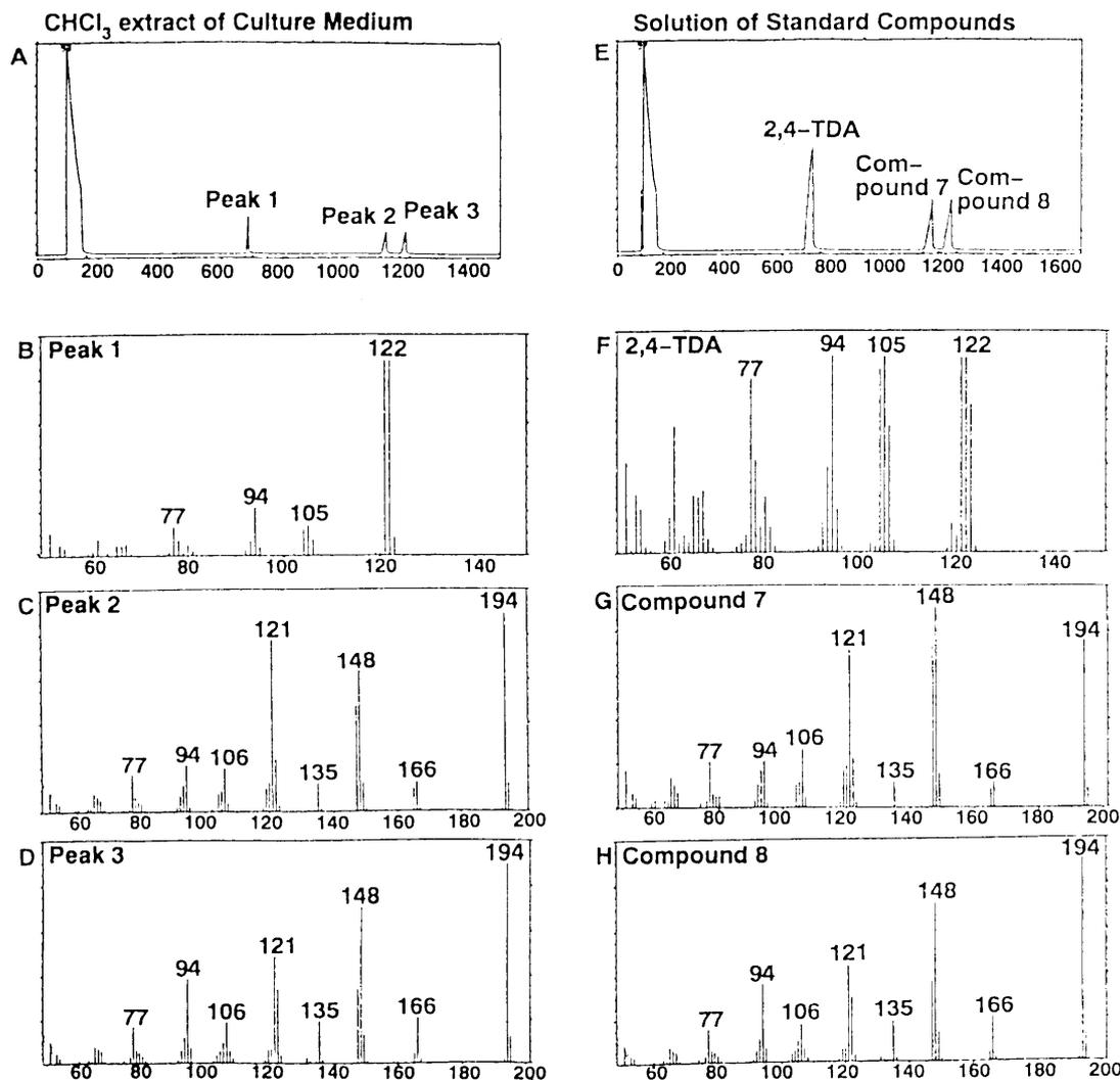
**Fig. 1.** GC-MS Analysis of the Products of Biodegradation of Toluene-2,4-dicarbamic Acid, Diethyl Ester (Compound 1) after 7 Days of Culture of *Exophiala jeanselmei* Strain REN-11A.
