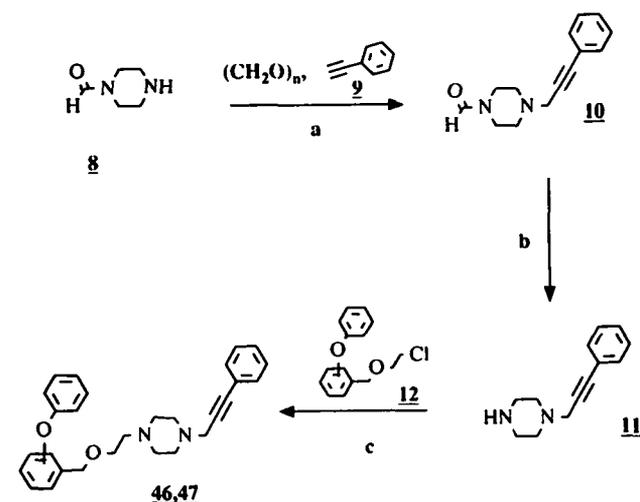
Scheme 2. Route 2: a) dioxane, reflux; b) 4N NaOH; c) K<sub>2</sub>CO<sub>3</sub>/KJ, 4-methyl-2-butan one.
