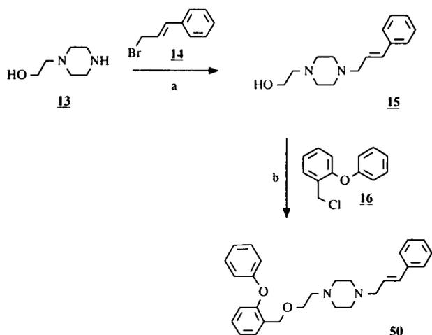
Scheme 4. Route 4: a) NaHCO<sub>3</sub>, dioxane, 85°C; b) KOC(CH<sub>3</sub>)<sub>3</sub>, DME, 40°C.
