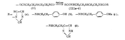
The desired product, bis(isocyanatoethyl) disulfide (II), was distilled in vacuum and identified by elemental analysis and IR spectroscopy. Bisisocyanate (II) was reacted with several biogenic amines and their derivatives, including imidazole, tyramine, O-methyltyramine, and histamine. The reaction was carried out with a stoichiometric ratio of the reagents in an inert organic solvent. The carbamide derivatives obtained (III) are given in Table 1.
