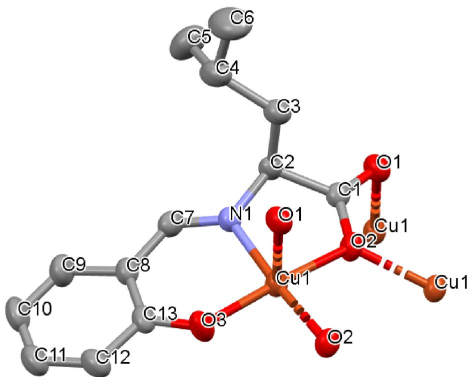
**Fig. 1.** Crystal structure of **1** as a product of microwave method. Hydrogen atoms are omitted for clarity. Selected bond distances ( $\text{\AA}$ ): Cu1–O3 = 1.880(4), Cu1–N1 = 1.923(5), dashed line Cu1–O2 (symmetry codes: 1-x, y-1/2, 2-z) = 1.982(4), Cu1–O2 = 2.012(4) (, and dashed line Cu1–O1 (symmetry codes: x, y-1, z) = 2.472(4)).
