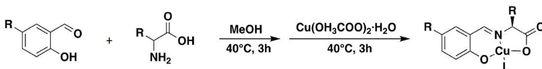
**Scheme 1.** Typical reaction scheme in a solution for the *L*-amino acid derivative Schiff base copper(II) complexes. In the case of microwave synthesis, 40 °C, 3 h are 85 °C, 20 min.
