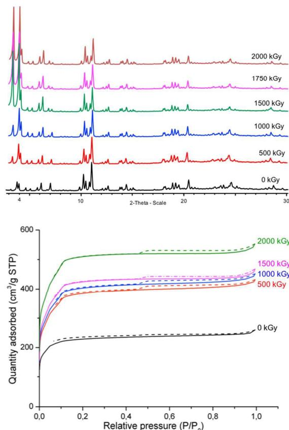
Figure 3. Influence of gamma irradiation doses (0–2 MGy) over as-synthesized MIL-100(Al): (bottom) Isotherm curves for the adsorption (solid) and desorption (dash) of nitrogen (77 K). (top) Powder X-ray diffractograms
