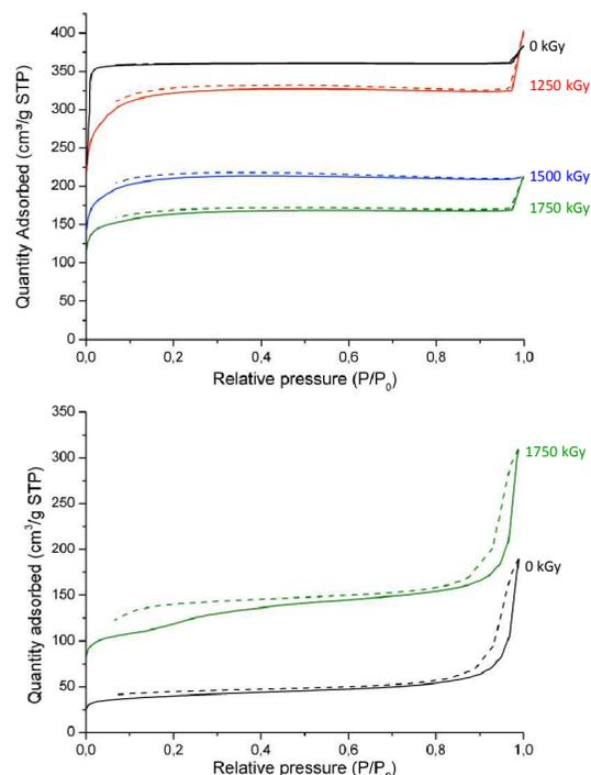
Figure 2. Isotherm curves for the adsorption (solid) and desorption (dash) of nitrogen (77K) in irradiated and non-irradiated ZIF-8 (top) and MIL-120 (bottom)
