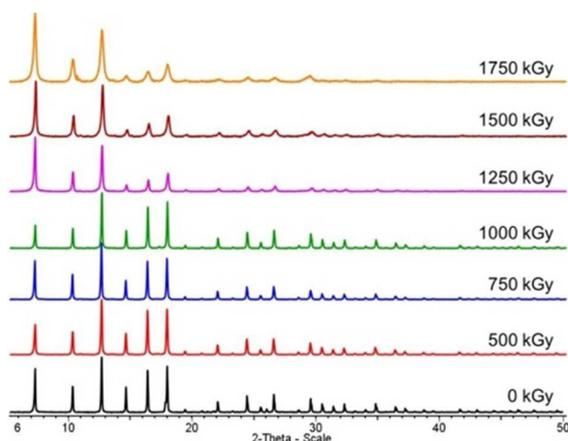
Figure 1. Evolution of powder X-ray diffraction patterns of non-irradiated and gamma irradiated zinc-based compound MOF ZIF-8 (copper wavelength) at different doses (0-1.75 MGy)
