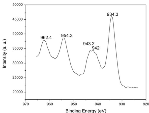
Figure 9 XPS deconvoluted spectra of Cu ( $2p_{3/2}$ ) of GLR-G2-Cu
