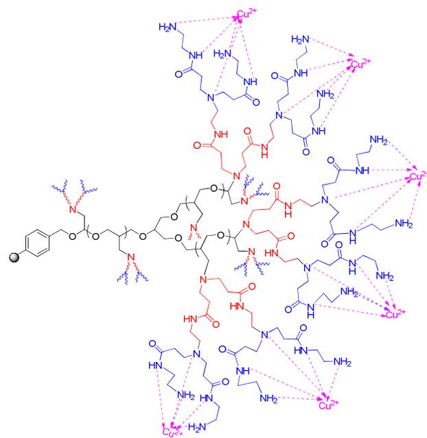
**Figure 6** Merrifield resin supported dendrigraft GLR-G2-Cu polymer having glycerol initiated PECH as core
