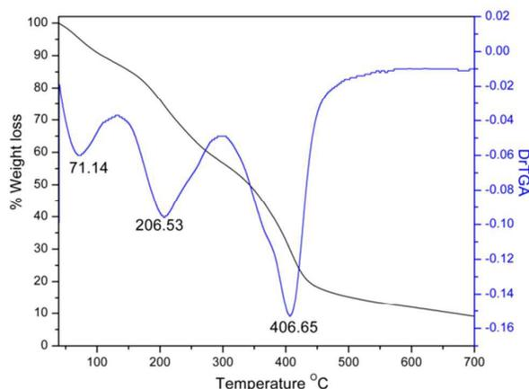
Figure 10 TG-DTG profile of GLR-G2-Cu
