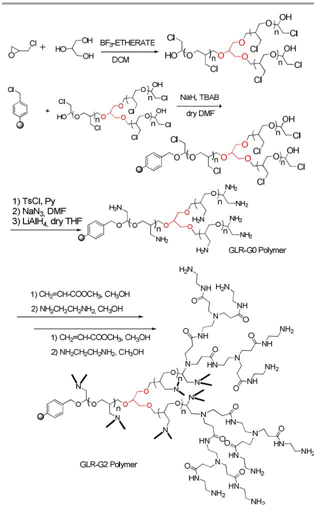
Scheme 1 Synthesis of GLR-G2 Dendrigrraft Polymer
