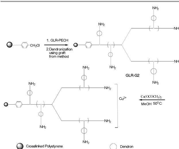
**Scheme 2** Synthesis of Merrifield resin supported dendrigraft GLR-G2-Cu polymer having glycerol initiated PECH as core.
