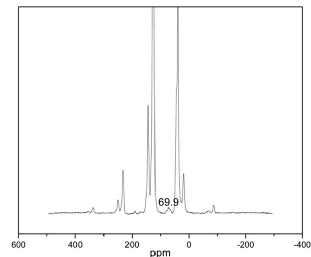
Figure 1 Solid state  $^{13}\text{C}$  NMR spectrum of PECH loaded Merrifield resin
