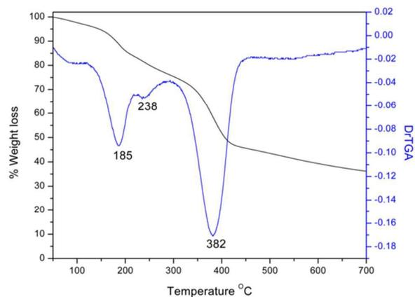
Figure 2 TG-DTG Profile of GLR-G0 Polymer
