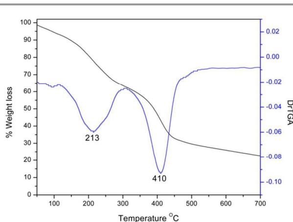
Figure 4 TG-DTG Profile of GLR-G1 Polymer
