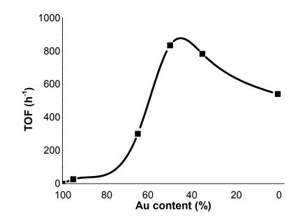
**Figure 9.** Au/Pd molar ratio effect in the CAL hydrogenation. Reaction conditions 100 °C, 1 H<sub>2</sub> bar, catalyst amount 50 mg, CAL 4 mmol, substrate/metal molar ratio 1200:1.
