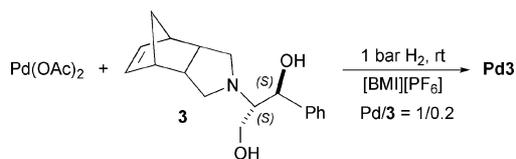
**Scheme 7** Synthesis of palladium nanoparticles containing ligand 3.
