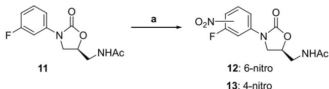
**Scheme 4.** Nitration of **11**. Reagents and conditions: (a)  $\text{KNO}_3$ ,  $\text{H}_2\text{SO}_4$ ,  $0^\circ\text{C}$  to rt, 4 h.
