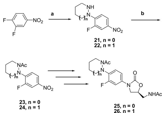
**Scheme 7.** Synthesis of **25** and **26**. Reagents and conditions: (a) *i*Pr<sub>2</sub>NEt, and pyrrolidine or hexahydro-pyridazine, CH<sub>3</sub>CN, 90 °C, 10 h; (b) Ac<sub>2</sub>O, pyridine, DMAP, THF, rt, 1 h.
