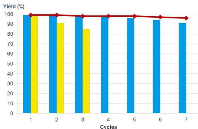
**Figure 6.** Catalysts recyclability. Performed with 1.5 mol% of complex 1 (yellow bars) or 2 (blue bars) under batch conditions, and by successive additions of substrate using complex 1 (red marks) with a final 0.16 mol% catalyst loading.
