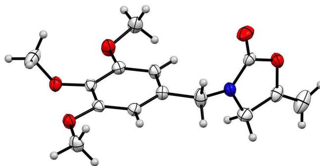
**Figure 5.** X-ray crystal structure (ORTEP representation) of **6k** at 45% thermal probability.<sup>[26]</sup>
