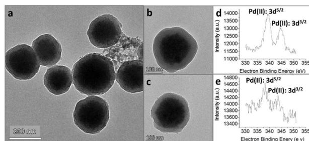
**Fig. 1** TEM images of SMNP@NHC-Pd **5**: (a) full image, (b) fresh prepared and (c) recovered single particle; XPS spectra of (d) fresh prepared and (e) recovered SMNP@NHC-Pd **5**.
