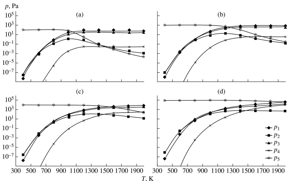
**Fig. 1.** Calculated temperature-dependent partial pressures in the Pb-I<sub>2</sub> system at total pressures of (a) 10<sup>2</sup>, (b) 10<sup>3</sup>, (c) 10<sup>4</sup>, and (d) 10<sup>5</sup> Pa;  $p_1$ – $p_5$  have the same meaning as in text.
