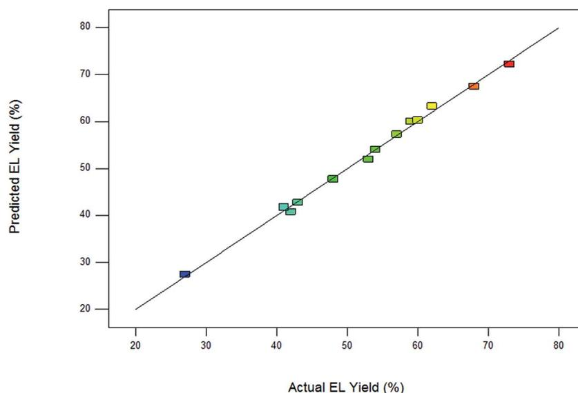
Fig. 5 Plot of actual versus predicted values of EL yield over Hierarchical-HZ-5 catalyst.
