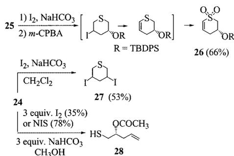
Scheme 7. Iodine-induced cyclization of 1-sulfanyl-4-pentene-2-ol derivatives **24** and **25**
