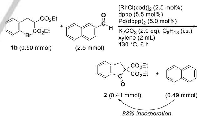
**Scheme 3.** Transfer Cyclocarbonylation of **1b** with 2-naphthalene.
