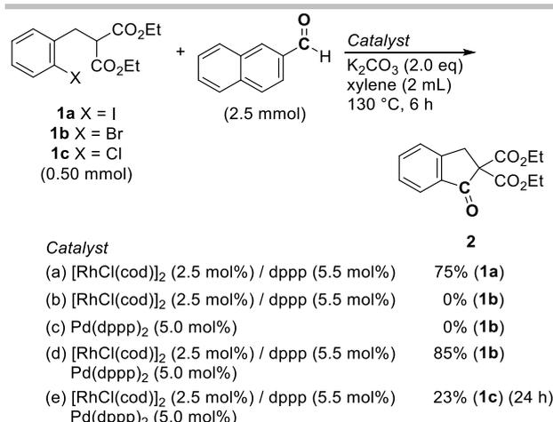
**Scheme 1.** Rh(I)/Pd(0)-Hybrid Catalyst Leads to Transfer Carbonylation of **1** with 2-naphthaldehyde.
