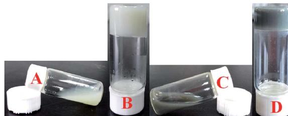
Fig. 3 Optical photograph of (A) mPEG-LUT/ $\alpha$ -CD sols before being converted to gels, (B) mPEG-LUT/ $\alpha$ -CD supramolecular hydrogels, (C) mPEG-LUT-Fe<sub>3</sub>O<sub>4</sub>/ $\alpha$ -CD sols before being converted to gels, and (D) mPEG-LUT-Fe<sub>3</sub>O<sub>4</sub>/ $\alpha$ -CD supramolecular hydrogels.
