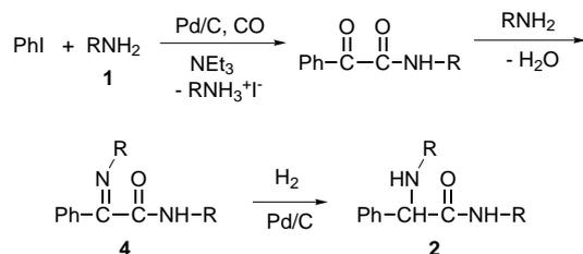
Scheme 1. Reaction pathway for the double carbohydroamination of iodobenzene. **a**: R = cyclohexyl, **b**: R = *n*-butyl, **c**: R = benzyl.
