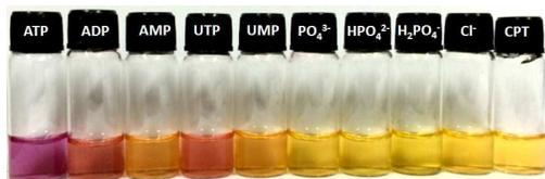
Fig. 2 Changes in the color of solutions of **CPT** (100  $\mu\text{M}$ ) in water induced by the addition of an equimolar amount of various anions.
