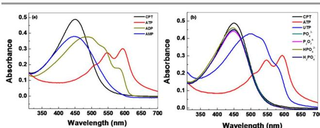
Fig. 3 Absorption spectra of **CPT** (100  $\mu\text{M}$ ) in water in the absence of anionic guest and (a) in the presence of an equimolar amount of ATP, ADP, or AMP, or (b) in the presence of an equimolar amount of ATP, UTP, or phosphate.
