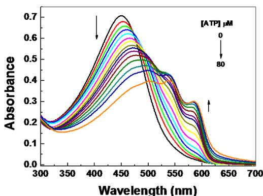
Fig. 1 UV-vis titration spectra of **CPT** (100  $\mu\text{M}$ ) in tris-HCl buffer solution with increasing amounts of ATP. [ATP] = 0, 4, 8, 12, 16, 20, 24, 28, 32, 36, 44, 52, 60, 68, 80  $\mu\text{M}$  from top to down.
