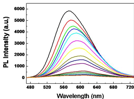
Fig. 4 Fluorescent titration spectra of CPT (100  $\mu\text{M}$ ) in tris-HCl buffer solution with different concentrations of ATP. [ATP] = 0, 2, 4, 6, 8, 10, 12, 14, 16, 18, 30, 40, 50, 70, 90  $\mu\text{M}$  from top to down.  $\lambda_{\text{ex}} = 450 \text{ nm}$ .
