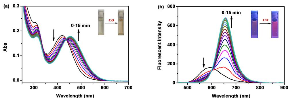
**Figure 1.** (a) UV-vis and (b) fluorescence spectral changes of the probe system ( $5 \mu\text{M}$  NIR-Ratio-CO +  $10 \mu\text{M}$  PdCl<sub>2</sub>) upon addition of CORM-3 ( $100 \mu\text{M}$ ) in PBS buffer ( $10 \text{ mM}$ , pH 7.4, 20% DMSO, v/v) at  $37^\circ\text{C}$ . For fluorescence measurement,  $\lambda_{\text{ex}} = 440 \text{ nm}$ , slit width:  $d_{\text{ex}} = d_{\text{em}} = 10 \text{ nm}$ . Inset: color changes and emission color changes under a portable 365 nm light.
