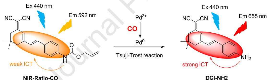
**Scheme 1.** NIR ratiometric fluorescent probe **NIR-Ratio-CO** for detection of CO.
