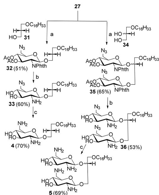
Scheme 3. Synthesis of compounds **4** and **5**. *Reagents and conditions:* (a) AgOTf, NIS, DCM, 3 h, rt (b) ethylenediamine/butanol (1:1), 90 °C, 2 h, rt (c) P(CH<sub>3</sub>)<sub>3</sub>, THF, H<sub>2</sub>O, 2 h, rt. Abbreviations: dichloromethane (DCM), 2,2, *N,N*-dimethylformamide (DMF), room temperature (rt) 23 °C, *N*-iodosuccinimide (NIS).
