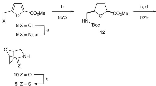
**Scheme 1** Reagents and conditions: (a)  $\text{Bu}_4\text{NN}_3$  (1.05 equiv), 2-MeTHF, r.t., 1.5 h, 98%; (b)  $\text{H}_2$ , 5% Rh/C (cat.),  $(\text{Boc})_2\text{O}$  (1.5 equiv), MeOH, 50 psi, r.t., 36 h; (c) aq 4 M HCl in 1,4-dioxane (4.0 equiv),  $\text{CH}_2\text{Cl}_2$ , r.t.; (d) NaOAc (1.5 equiv), butan-2-ol, 100 °C, 3 h; (e) Lawesson's reagent, toluene, 90 °C, 1.5 h, 93%.
