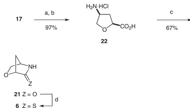
**Scheme 5** Reagents and conditions: (a) LiOH·H<sub>2</sub>O (7.0 equiv), THF–MeOH–H<sub>2</sub>O (6:3:1), r.t., 1 h; (b) aq 3 M HCl, 70 °C, 1 h; (c) DCC (1.0 equiv), pyridine (3.0 equiv), MeCN, reflux, 1 h; (d) Lawesson's reagent, toluene, 90 °C, 1 h, 74%.
