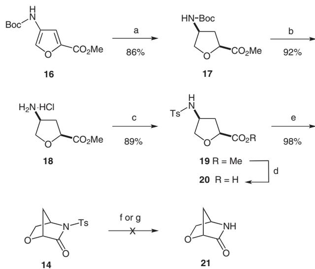
**Scheme 4** Reagents and conditions: (a) 5% Rh/C, MeOH, 50 psi, r.t., 36 h; (b) aq 4 M HCl in 1,4-dioxane (4.0 equiv), CH<sub>2</sub>Cl<sub>2</sub>, r.t., 1 h; (c) TsCl (1.0 equiv), Et<sub>3</sub>N (2.0 equiv), CH<sub>2</sub>Cl<sub>2</sub>, 24 h; (d) LiOH·H<sub>2</sub>O (7.0 equiv), THF–MeOH–H<sub>2</sub>O (6:3:1), r.t., 1 h; (e) Ac<sub>2</sub>O, NaOAc (10 equiv), reflux, 2 h; (f) Na, naphthalene, DME, –78 °C, 30 min; (g) Li, NH<sub>3</sub>, –78 °C, 30 min.
