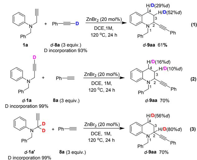
**Scheme 4.** Deuterium labeling study for the intramolecular hydroarylation-redox CDC reaction of *N*-propargylanilines and phenylacetylenes.
