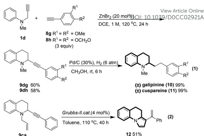
**Scheme 3.** Synthesis of natural alkaloids and important intermediate.
