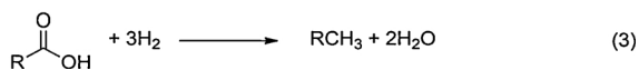
Scheme 1. Conversion of fatty acids to alkanes via decarboxylation (Path 1) or decarbonylation (Path 2), abbreviated collectively as DCOx, or hydrodeoxygenation (HDO) (Path 3).
