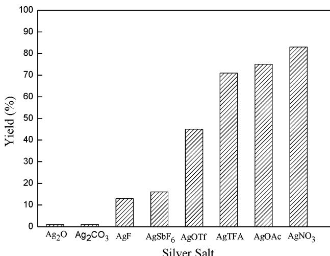
Figure 1. The effect of various silver salts. Reaction conditions: **1a** (0.5 mmol), **2a** (3.0 mmol),  $\text{Pd}(\text{OAc})_2$  (0.025 mmol), silver salt (1.0 mmol),  $\text{Na}_2\text{HPO}_4$  (1.0 mmol), DMSO (1.0 mL),  $\text{H}_2\text{O}$  (0.5 mL), 75°C, 20 h.
