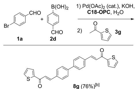
[a] Reaction conditions: 1) 4-bromobenzaldehyde (**1a**; 0.27 mmol), (4-formylphenyl)boronic acid (**2d**; 0.32 mmol), Pd(OAc)<sub>2</sub> (3 mol-%), KOH (10.75 equiv.), C18-OPC (0.75 equiv.), H<sub>2</sub>O (4 mL), 80 °C, 2 h; 2) 2-acetylthiophene (**3g**; 0.59 mmol), 80 °C, 5 h. [b] Yield determined by GC–MS (internal standard).
