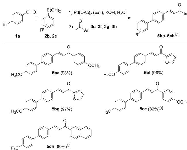
[a] Reaction conditions: 1) 4-bromobenzaldehyde (**1a**; 0.27 mmol), arylboronic acid **2b** or **2c** (0.32 mmol), Pd(OAc)<sub>2</sub> (3 mol-%), KOH (6 equiv.), H<sub>2</sub>O (3 mL), 80 °C, 1 h; 2) aromatic ketone **3c**, **3f**, **3g**, or **3h** (0.30 mmol), 80 °C, 5 h. [b] Yield determined by GC–MS (internal standard). [c] C18-OPC (0.5 equiv.) and KOH (6.5 equiv.) were used for 2 h in the first step.
