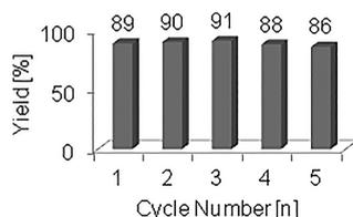
Figure 2. Recycling of the Pd/C18-OPC/H<sub>2</sub>O system in the synthesis of biaryl-chalcone **6af**.
