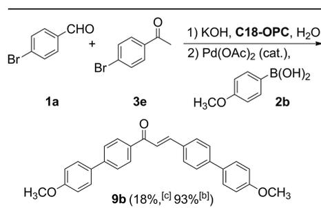
[a] Reaction conditions: 1) 4-bromobenzaldehyde (**1a**; 0.27 mmol), 4-bromoacetophenone (**3e**; 0.30 mmol), KOH (8.75 equiv.), C18-OPC (0.75 equiv.), H<sub>2</sub>O (5 mL), 80 °C, 2 h; 2) (4-methoxyphenyl)boronic acid (**2b**; 0.65 mmol), Pd(OAc)<sub>2</sub> (6 mol-%), 80 °C, 2 h. [b] Yield determined by GC–MS (internal standard). [c] One-pot, 80 °C, 4 h.
