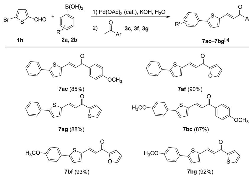
[a] Reaction conditions: 1) 5-bromo-2-thiophenecarbaldehyde (**1h**; 0.26 mmol), arylboronic acid **2a** or **2b** (0.31 mmol), Pd(OAc)<sub>2</sub> (3 mol-%), KOH (6 equiv.), H<sub>2</sub>O (3 mL), 80 °C, 1 h; 2) aromatic ketone **3c**, **3f**, or **3g** (0.29 mmol), 80 °C, 5 h. [b] Yield determined by GC–MS (internal standard).
