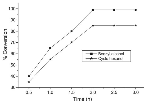
Fig. 3. Catalytic oxidation of benzylalcohol and cyclohexanol in different time intervals.
