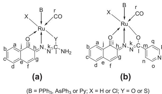
Fig. 2. Structure of complexes.
