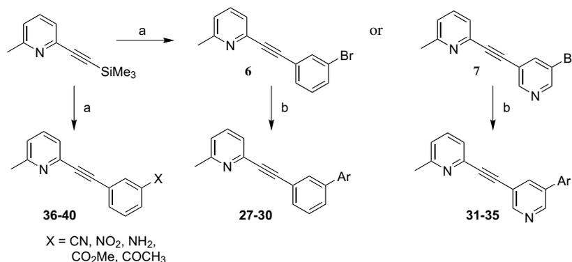
**Scheme 3.** Reagents and conditions: (a) aryl or heteroaryl bromide, CuI, PdCl<sub>2</sub>(PPh<sub>3</sub>)<sub>2</sub>, Et<sub>3</sub>N, Bu<sub>4</sub>NF, DMF, 70 °C; (b) aryltrialkylstannane, Pd(PPh<sub>3</sub>)<sub>4</sub>, toluene, reflux.
