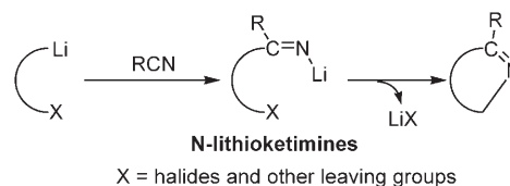
Scheme 1. The conventional way to nitrogen-containing heterocycles from N -lithioketimines generated from organolithium reagents and nitriles.
