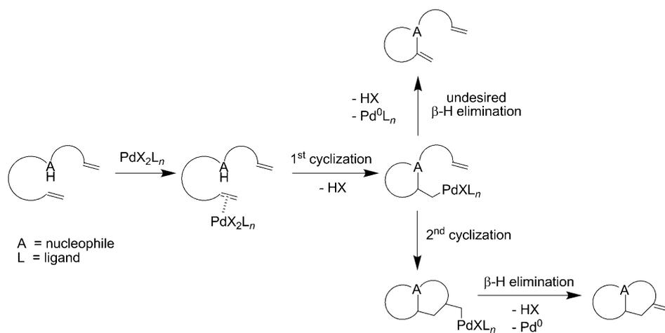
Scheme 5. Midway  $\beta$ -hydride elimination disrupting oxidative cascade cyclization.
