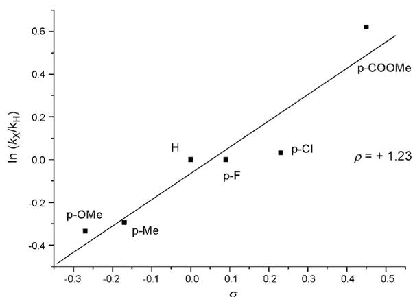
Figure 1. Hammett plot for Pd<sup>II</sup>-catalyzed oxidative cascade cyclizations.
