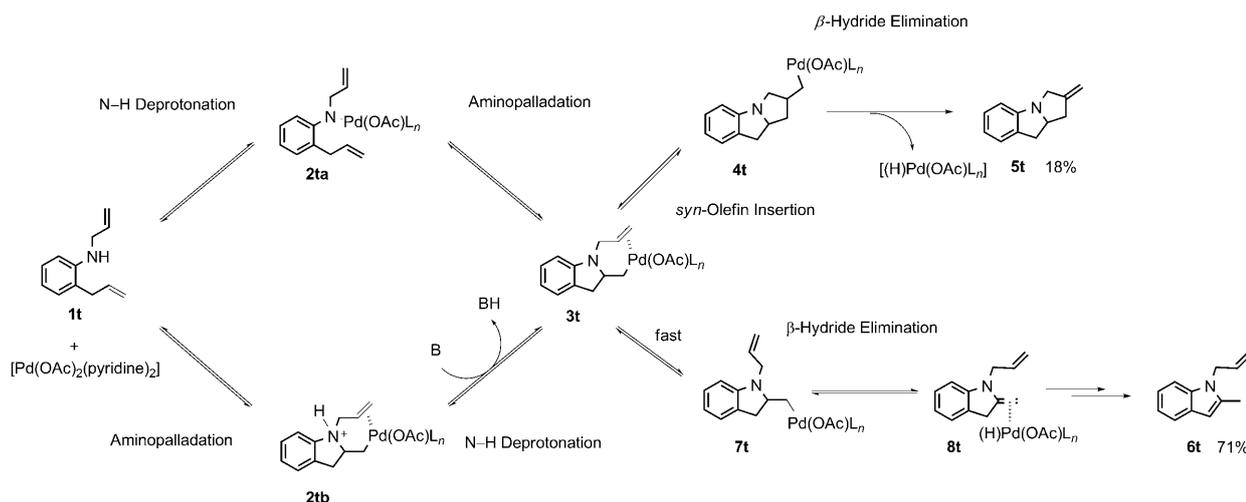
Scheme 10. Mechanistic pathways of the cascade cyclization of **1t**.
