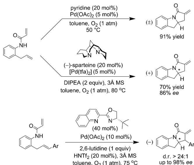
Scheme 2. Palladium-catalyzed oxidative cascade cyclization reactions. DIPEA = *N,N*-diisopropylethylamine.
