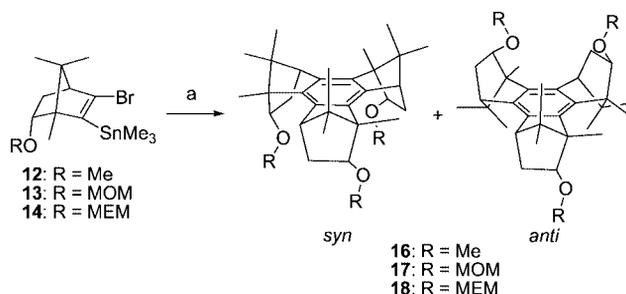
Scheme 8. Synthesis of cyclotrimers **16**, **17**, **18**. Reagents and conditions: a) CuTC, NMP, 0 °C to room temperature [*syn*-**16** (78%), *syn*-**17** (72%), *syn*-**18** (77%)].
