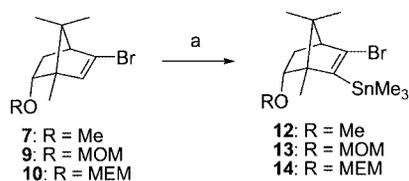
Scheme 6. Stannylation of protected bornenols **7**, **9**, **10**. Reagents and conditions: a) i) LDA, THF, room temperature; ii)  $\text{Me}_3\text{SnCl}$  (83, 86, 93%).
