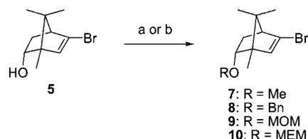
Scheme 4. Protection of the bromobornenol **5**. Reagents and conditions: a) i)  $\text{NaH}$ ,  $\text{Et}_2\text{O}$ ,  $0^\circ\text{C}$ ; ii)  $\text{MeI}$  or  $\text{BnBr}$  (80 or 74%); b)  $\text{MOMCl}$  or  $\text{MEMCl}$ ,  $i\text{Pr}_2\text{NEt}$ ,  $\text{CH}_2\text{Cl}_2$ , room temperature (95 or 92%).
