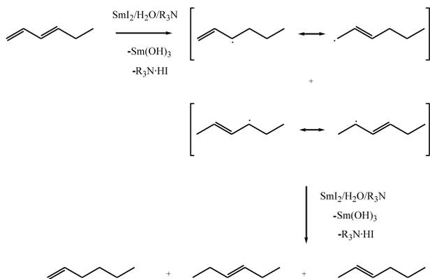
**Scheme 1.** Suggested mechanism for the reduction of 1,3-hexadiene.
