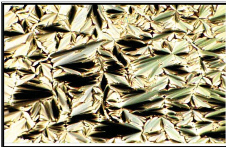
**Figure 5.** Mesophase texture of the SmA phase obtained on cooling. A typical focal-conic fan texture (200 $\times$  magnification) for the compound [VI<sub>7</sub>] at 120°C.
