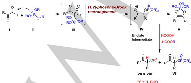
**Scheme 5.** Plausible reaction mechanism for the synthesis of  $\alpha$ -phosponyloxy ketone
