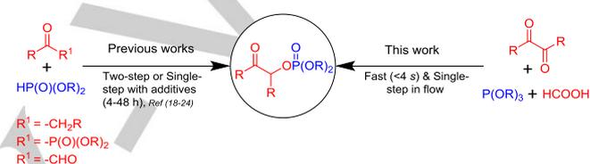
**Scheme 1.** Comparative approaches for the synthesis of  $\alpha$ -phosphonyloxy ketones between the reported work and our work.
