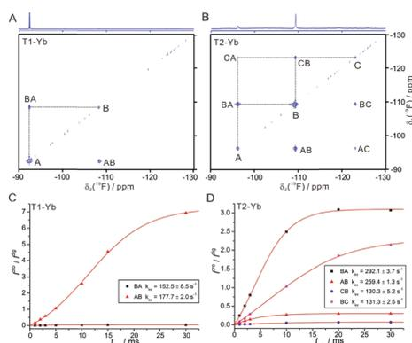
**Fig. 3** Exchange rates between different isomers determined by 2D <sup>19</sup>F-EXSY spectra for the DOTA-Ln complexes. The <sup>19</sup>F-EXSY spectra: (A) T1-Yb, and (B) T2-Yb. The exchange rates between different isomers: (C) T1-Yb, and (D) T2-Yb. The NMR spectra were recorded for the 20 mM lanthanide complex with a mixing time of 20 ms.
