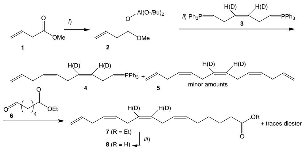
Scheme 2. Preparation of 6Z,9Z,12Z,15-hexadecatetraenoic acid (**8**). (i) DIBAL-H, (ii) from **11** by deprotonation with 2.2 equivalents of  $\text{KN}(\text{SiMe}_3)_2$ , (iii) LiOH/THF/H<sub>2</sub>O.
