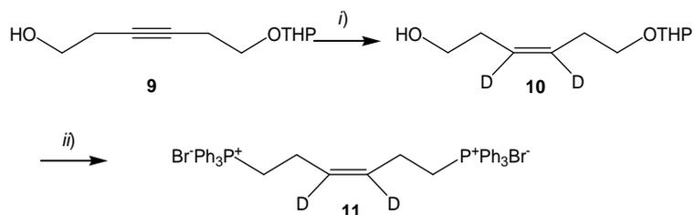
Scheme 3. Preparation of [3,4-<sup>2</sup>H<sub>2</sub>]-(*Z*)-hex-3-enyl-1,6-bis-[triphenylphosphonium bromide] (**11**). (i) P-2-Ni/D<sub>2</sub>, (ii) 1: Br<sub>2</sub>, PPh<sub>3</sub>; 2: PPh<sub>3</sub> reflux.
